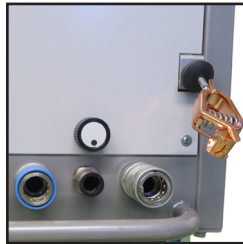
Integrated grounding roll for more safety
