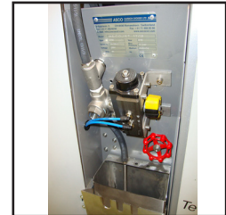
Box for additive with approx. 5 kg (11.02 lb) capacity
