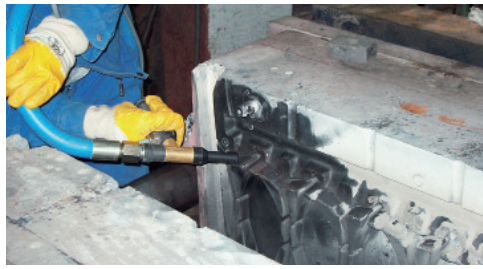
Cleaning of a hotingot mould without dismantling
